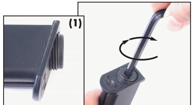
• Screw the bottom of the magazine. When pressure starts increasing in the magazine (expansion of the CO2 in the magazine can be heard), finishing screwing rapidly. Very important : do not tighten excessively, it could permanently damage the O'rings (picture 1). Take care to put the screw in the right position as shown on the picture.
